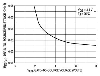
Figure 5. On–Resistance versus Gate–to–Source Voltage
