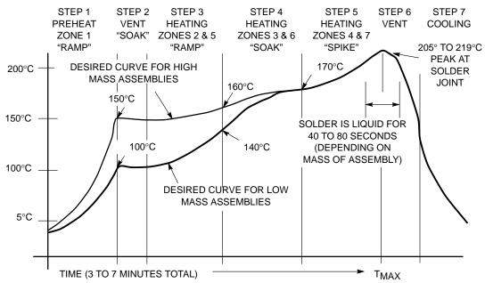
Figure 17. Typical Solder Heating Profile
