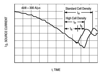
Figure 13. Reverse Recovery Time (t<sub>rr</sub>)
