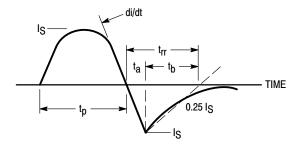
Figure 16. Diode Reverse Recovery Waveform
