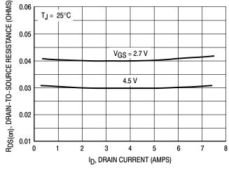
Figure 6. On–Resistance versus Drain Current and Gate Voltage
