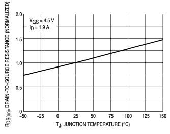
Figure 7. On–Resistance Variation with Temperature
