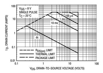
Figure 14. Maximum Rated Forward Biased Safe Operating Area
