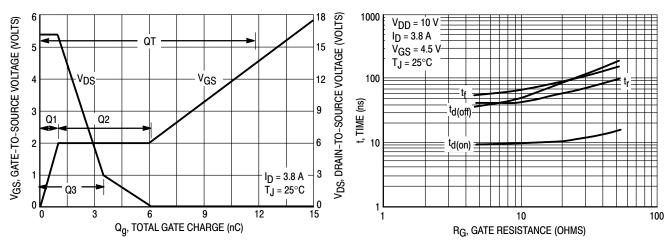
Figure 10. Gate-To-Source and Drain-To-Source Voltage versus Total Charge
