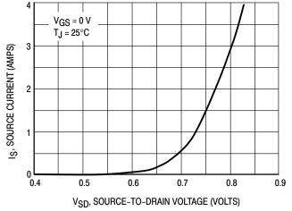
Figure 12. Diode Forward Voltage versus Current
