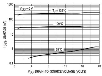
Figure 8. Drain-to-Source Leakage Current versus Voltage
