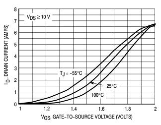
Figure 4. Transfer Characteristics
